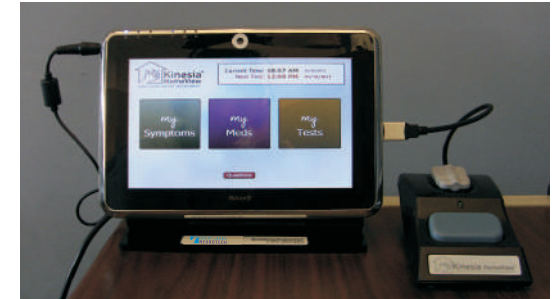
Figure 5: Incorporating a docking station and minimizing the amount of information on the software encourages correct patient use. Additionally, a touch-screen PC with large buttons is important when designing a home monitor for patients with movement disorders.
