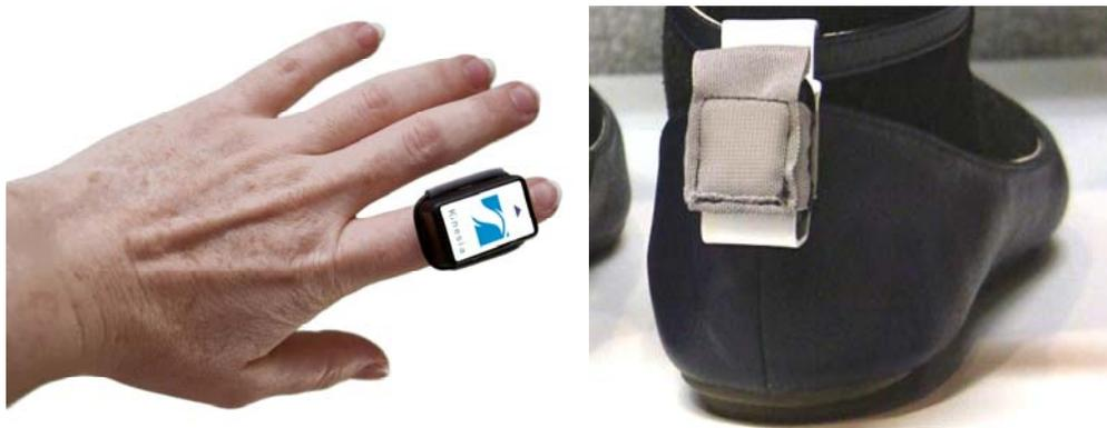
**Figure 2: Kinesia HomeView Sensor Positioning**
