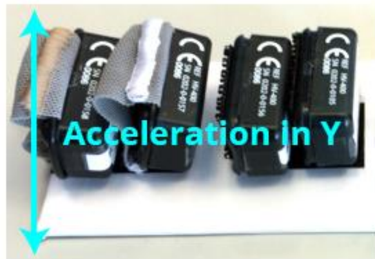
Figure 2. Example of the shake/perturbation test with the potential setup shown on the left and collected data on the right. The time of the peaks can be used to align the times of the sensor data.
