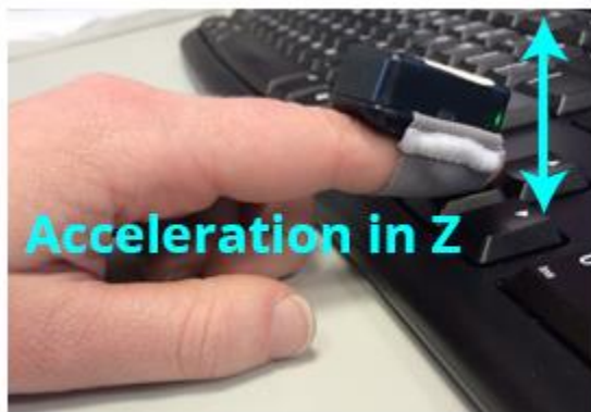
Figure 3. Example of the computer synchronization test with the potential setup for a keyboard shown on the left and collected mouse and sensor data on the right. The settled sensor acceleration time can be compared to the time of the state change to evaluate the delay between the sensor and computer.
