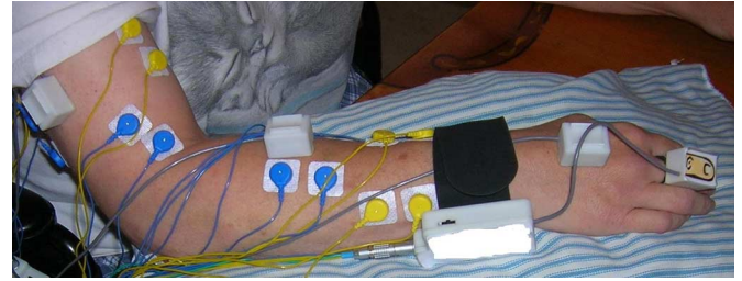
Fig. 1. Each subject was setup with six KinetiSense motion and EMG capture systems consisting of a sensor unit and command module connected by a thin cable.
