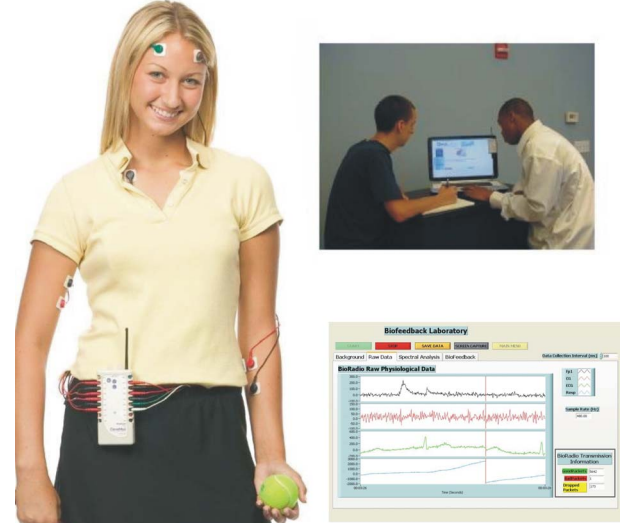
Fig. 1. The CleveLabs biomedical engineering laboratory system integrates wireless biotechnology for data acquisition with application-based software to optimize the student laboratory experience.
