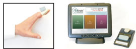
Figure 1. Kinesia HomeView includes a wireless finger-worn sensor unit (left) and a touch screen tablet PC with a USB docking station for the sensor unit (right).
