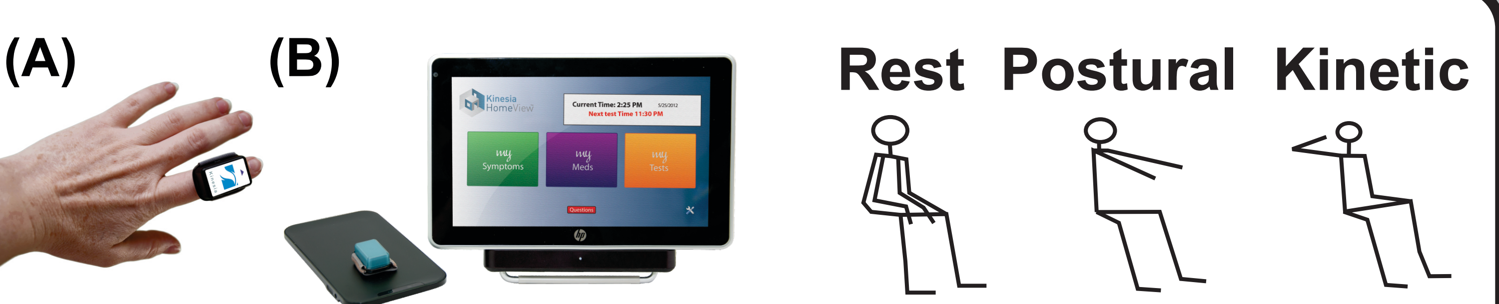
Figure 1. The Kinesia HomeView system includes a wireless finger-worn sensor unit (A) and a touch-screen tablet PC with a wireless inductive charging pad for the sensor unit (B).
