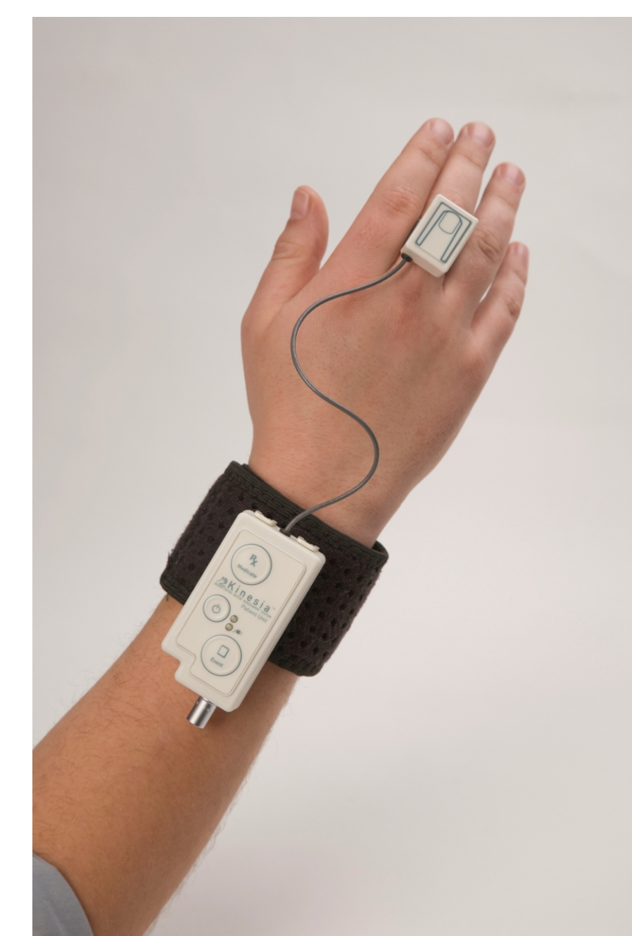
Figure 1. Kinesia™ consists of a finger worn sensor unit that contains accelerometers and gyroscopes, and a wrist worn command module that wirelessly transmits data to a computer.
