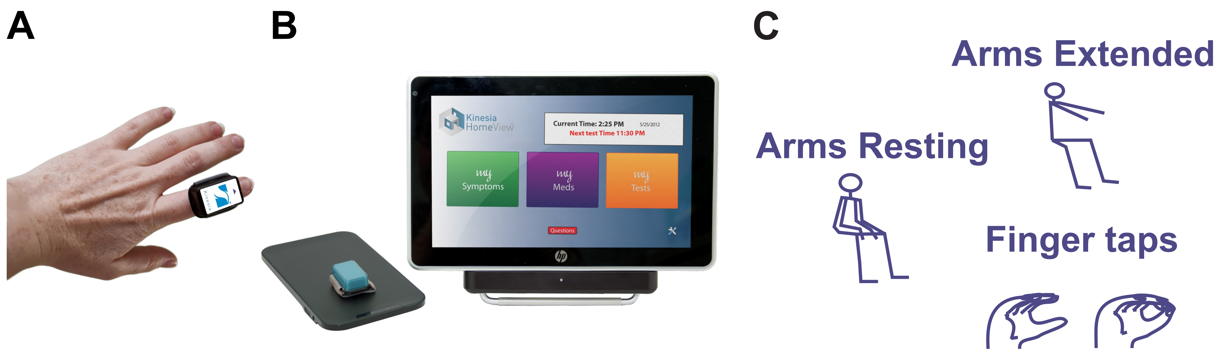
Figure 1. Kinesia includes a wireless finger-worn motion-sensor unit (A) and a touch screen tablet PC with inductive charge (B). The automated motor assessment included three 15-second tasks (C). The first two tasks were assessments of rest and postural tremor, while the third task involved repetitive finger tapping to evaluate bradykinesia (speed), hypokinesia (amplitude), and dysrhythmia (rhythm).
